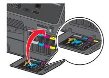
Behind the ink cartridge access door, you will find the customer support label, which contains the ink cartridge information, model number, product Web site, and customer support number.
